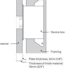
Medium: Install the device box 22mm (0.87") away from finished wall surface.
