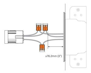
6. Measure and drill hole locations in your finish material. The reveal size must be at least 36.5mm (1.4375") diameter.
