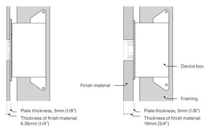
**Short:** Install the device box 9.5mm (0.37") away from finished wall surface.
