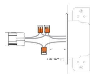
5. Measure and drill hole locations in your finish material. The reveal size must be at least 36.5mm (1.4375") diameter.
