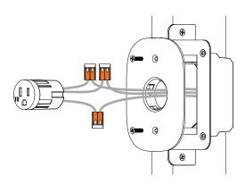
If a wet material such as grout, mortar, plaster etc is used, use the trim cap (22.1.2) to block the face of the devices to create the necessary reveal. It is recommended to use a Medium barrel for these applications.
