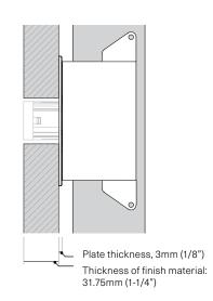
Long: Install the device box 35mm (1.35") away from finished wall surface.
