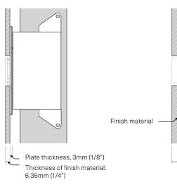
Short: Install the device box 9.5mm (0.37") away from finished wall surface.
